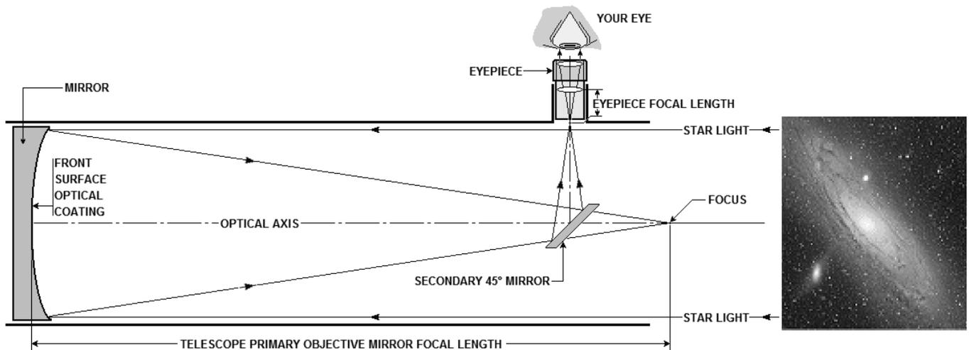
Newtonian Telescope Function: Above is a cross-sectional view of the Newtonian Telescope tube. The scope consists of a tube, in which is mounted a Curved Primary Objective Mirror at the bottom (the curve is a parabola.) Up at the top end of the tube is a smaller Flat Mirror set at 45° to the Optical Axis of the Primary Mirror, along with a mounting on the side of the tube designed for holding interchangeable eyepieces. (Different eyepieces provide differing magnifications.)
